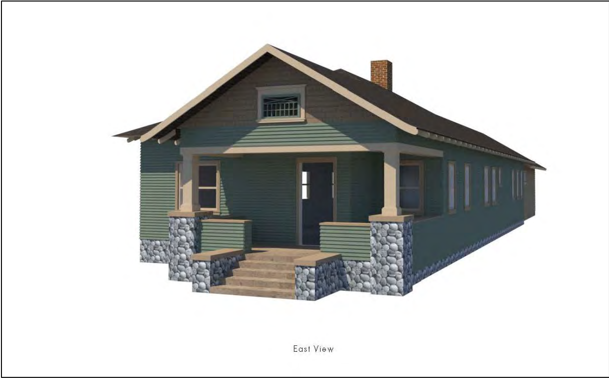
Figure 7: Renderings East Elevation *original volume of historic house appears in green; addition appears in beige
