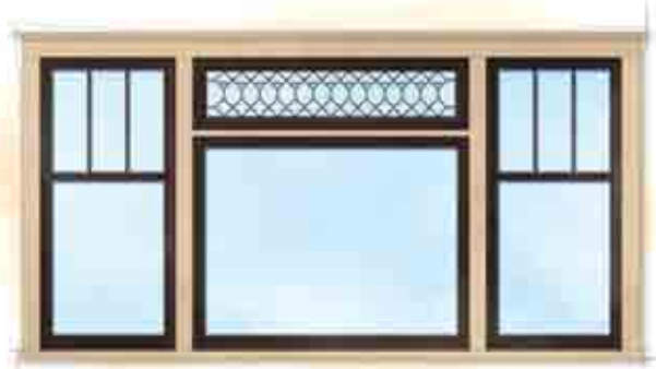
Casement, picture and transom window combination (exterior)
