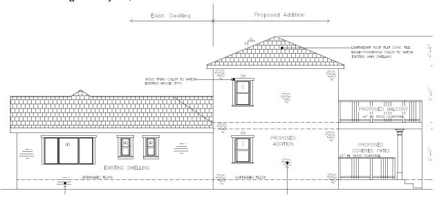
The changes to the south elevation include; a new window on the second floor, the installation of wood siding for the first floor, a new transitional strip between existing and proposed, a transitional strip between stucco and wood siding, and the reduction of the building height of the proposed addition. With the added materials, the new design helps lesson the empty wall space on the elevation, as requested by the Commission.
