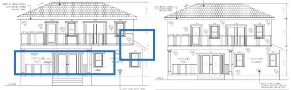
The rear elevations changes include exterior 8-inch wood siding to the first floor and changes to the roof illustration on the north-facing wall, to accurately represent the first floor roof pitch and height.
