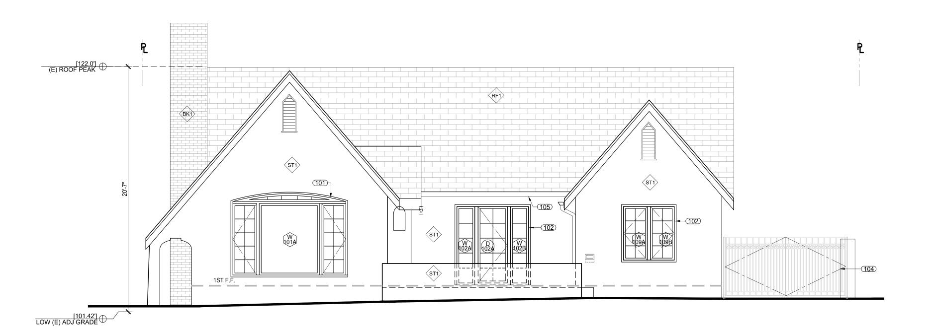
SCOPE OF WORK BY ELEVATION - NO SIGNIFICANT CHANGE TO THIS STREET FACING ELEVATION - REPAIRS TO EXISTING WOOD ARCHED WINDOW - REPLACEMENT OF REMAINING WINDOWS - REPAIRS TO DAMAGED EAVE FACIA BOARDS - REPLACE WROUGHT IRON GATE - REPAINT HOUSE - RE-ROOF
