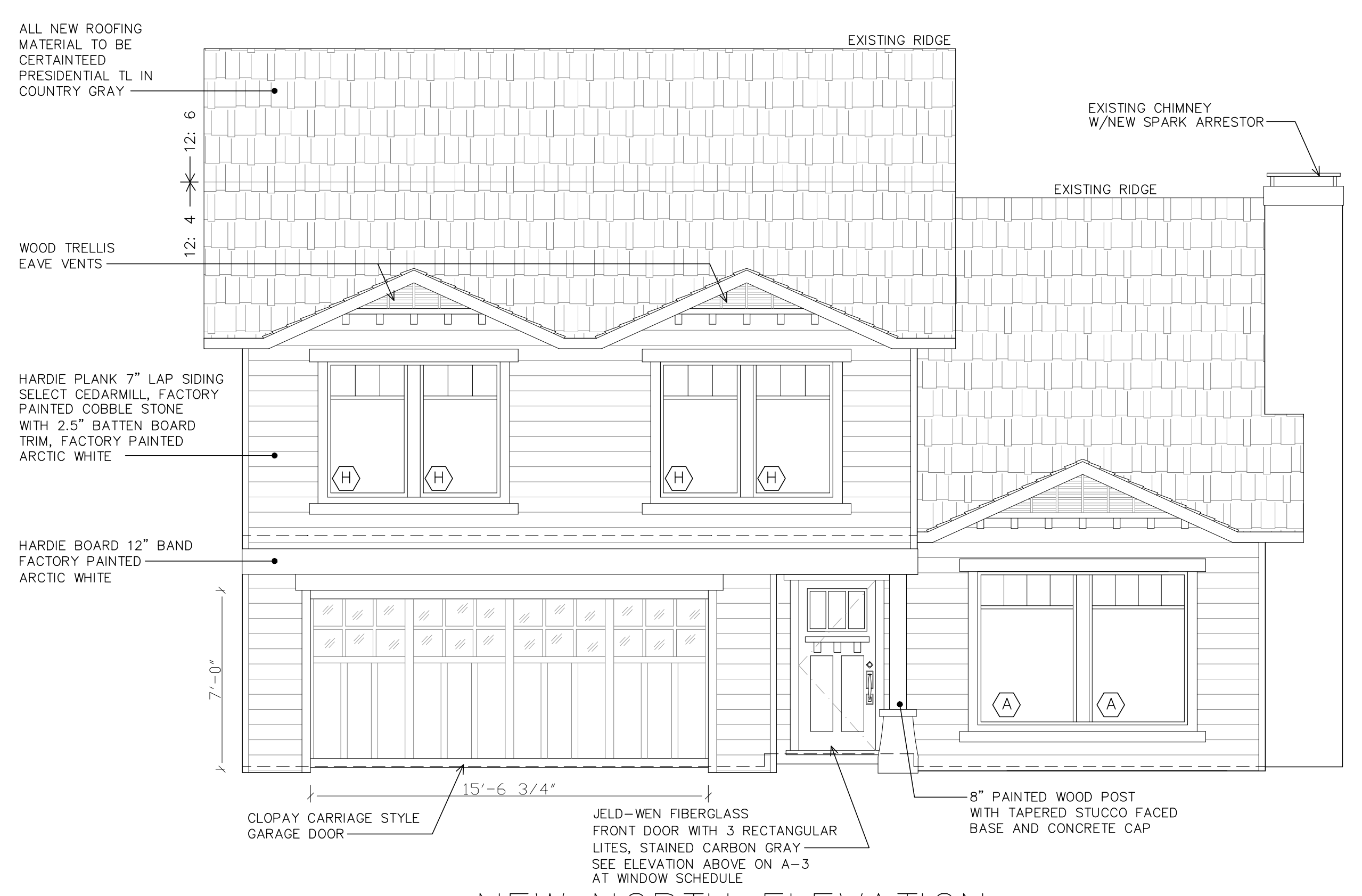
2 A-5 1/4" = 1'-0" NEW NORTH ELEVATION
