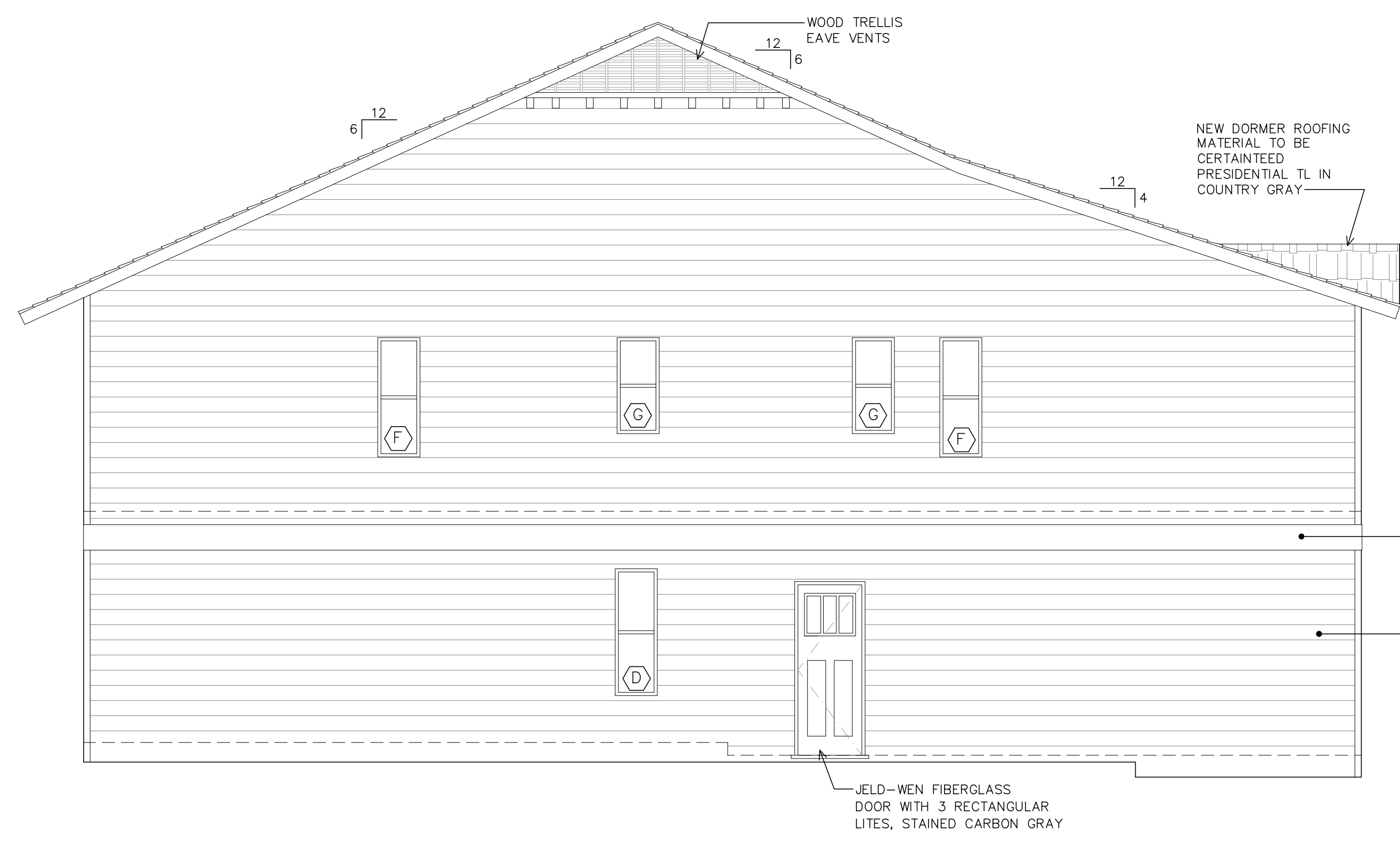
2 A-6 1/4" = 1'-0" NEW EAST ELEVATION
