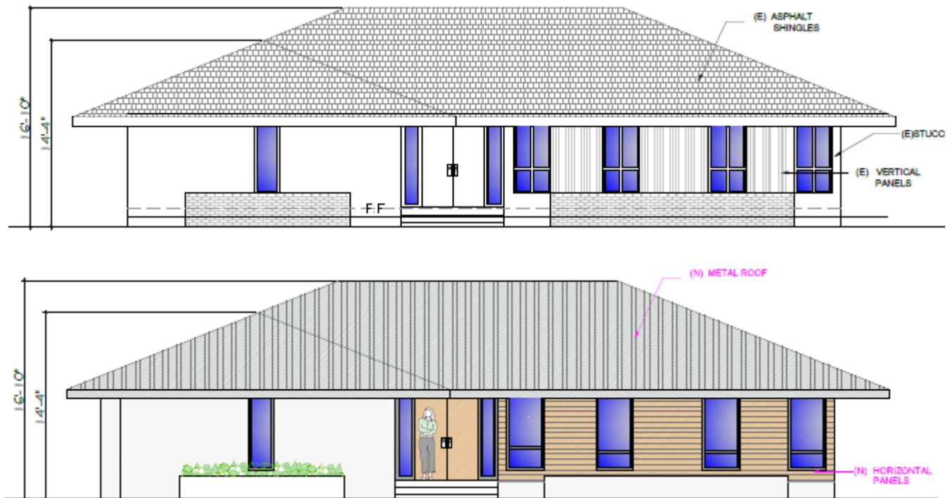
Figure 4: Existing & Proposed South Elevation (Front)
