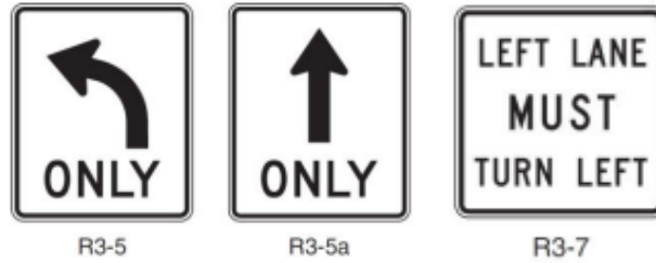
Figure 4: Mandatory Movement Lane Control Signs
