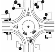
most appropriate for new developments or redevelopment areas. Roundabouts have an insignificant affect in reducing traffic speeds, but serve to allocate rightof-way at an intersection similar to a traffic signal.
