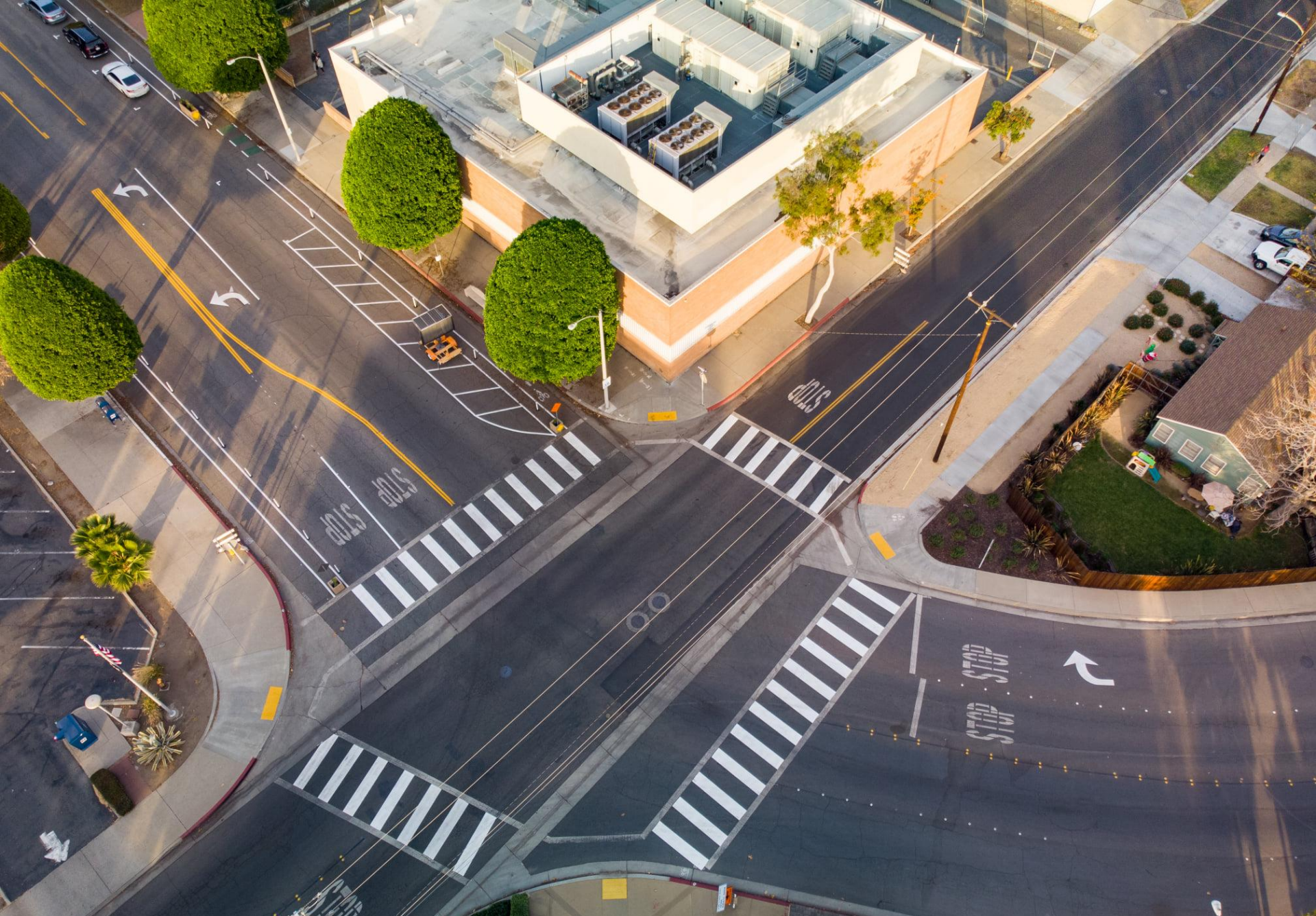
Demo of High-Vis Crosswalks, Curb Extensions, Protected Rollway - Glendora, CA (2020)
