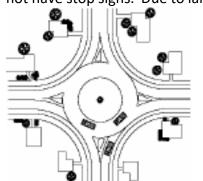
most appropriate for new developments or redevelopment areas. Roundabouts have an insignificant affect in reducing traffic speeds, but serve to allocate right-of-way at an intersection similar to a traffic signal.
