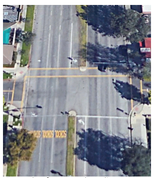
Example of proposed median trimming location at intersection of Fair Oaks Avenue & Banks Street
