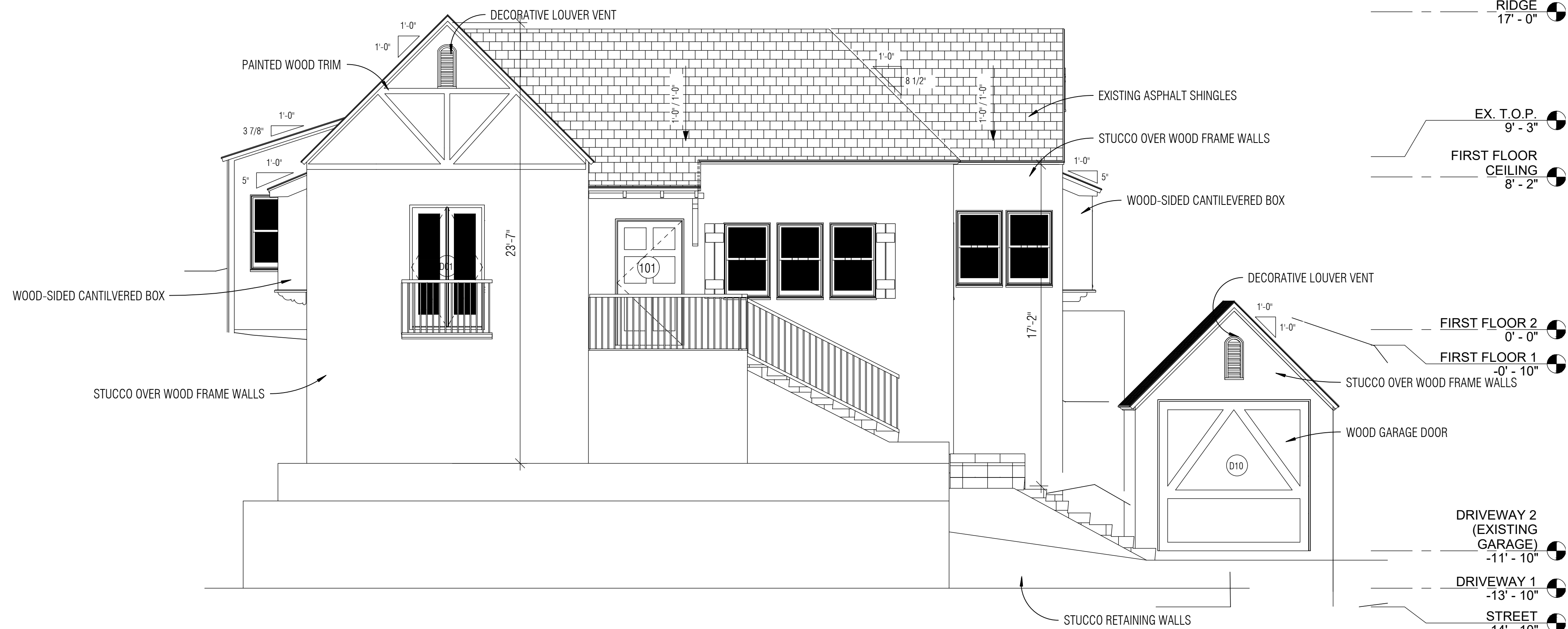
① EXISTING WEST ELEVATION (Front) 1/4" = 1'-0"
