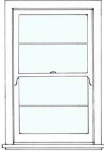
Two-over-two (multi-light) double-hung window
