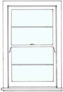
Two-over-two (multi-light) double-hung window
