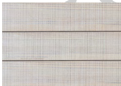
EGRET EXTERIOR CLADDING & INTERIOR WALL/CEILING CLADDING (WEATHERED 2 MONTHS)
