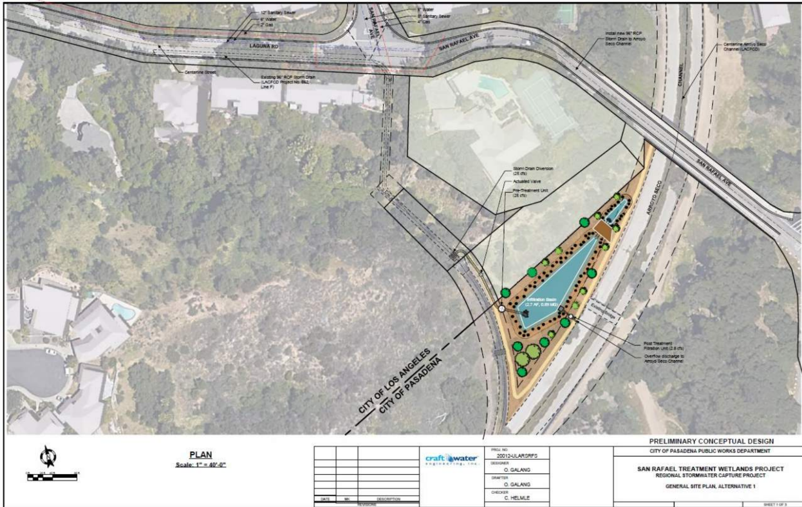
Figure 2. Preliminary concept schematic for the San Rafael Infiltration Basin BMP, east of San Rafael Creek (may not represent final project details).
