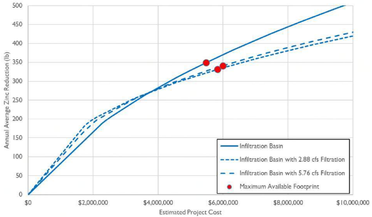
Figure 8. Comparison of infiltration basin results with and without filtration.
