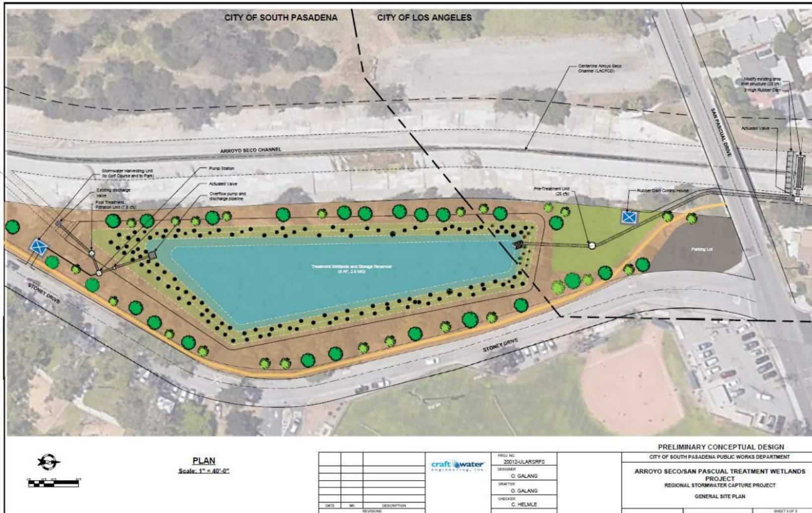
Figure 2. Preliminary concept schematic for the San Pascual Treatment Wetlands BMP as a treatment wetland, east of the Arroyo Seco Channel (may not represent final project details).
