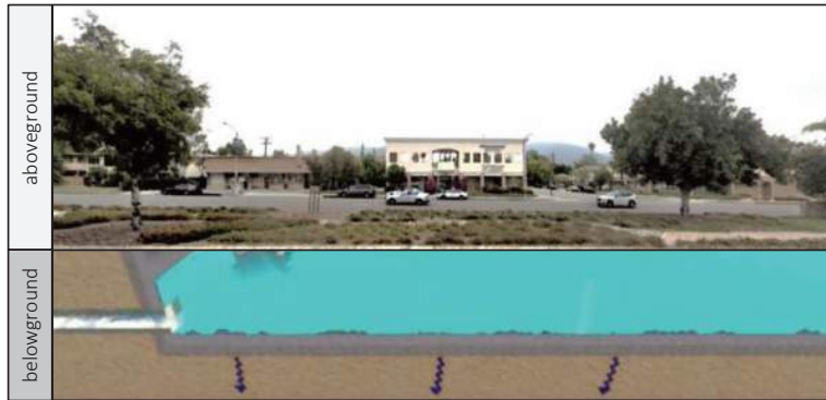
Underground regional infiltration system below a street median
