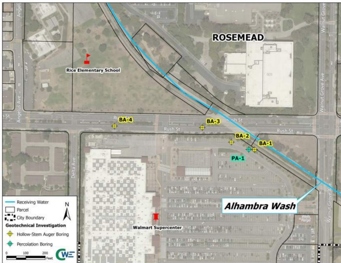
Figure 3-7 Boring Sites at Alhambra Wash
