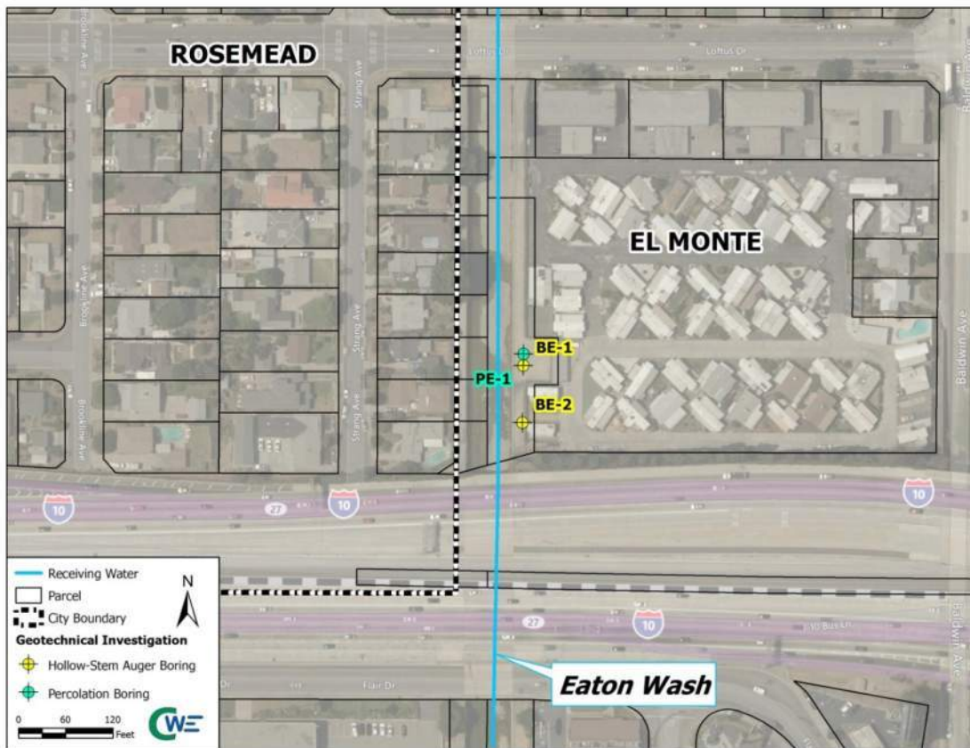
Figure 3-8 Boring Sites at Eaton Wash
