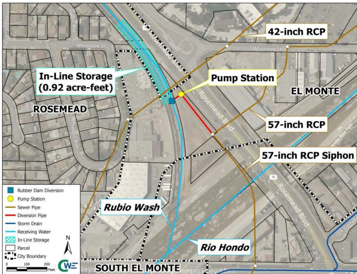
Figure 4-7 Rubio Wash Alternative R2: In-Line Storage
