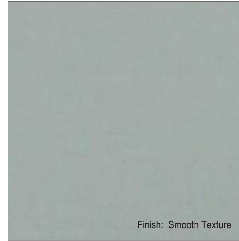
Steel troweled plaster, 40 Dove Gray integral color, La Habra or other, Fry Reglet "V" plaster reveals where required.
