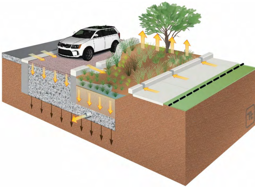
Illustration of a green street (arrows indicate water pathways)
