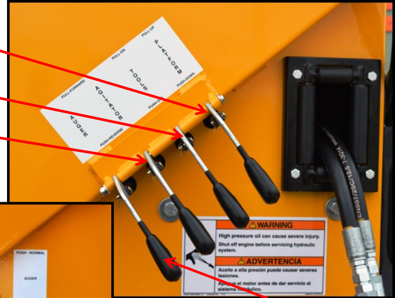
Auger Controls "On" "Forward / Reverse"
