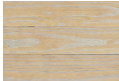
MANAWATU EXTERIOR CLADDING (WEATHERED 2 MONTHS)
