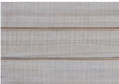
PATINA EXTERIOR CLADDING (WEATHERED 2 MONTHS)
