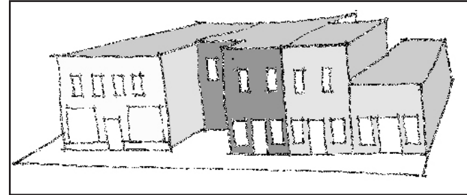
This infill construction does not respect the "streetwall."
