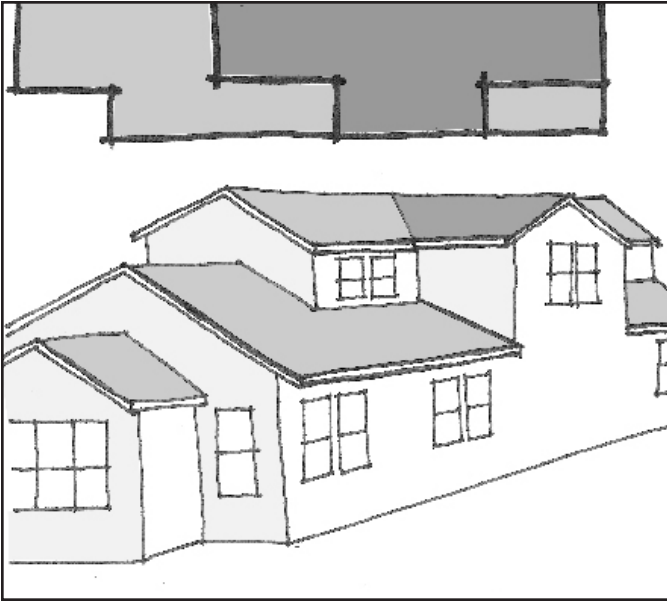
This diagram illustrates that varying the rooflines of the building can help to break up the massing of an addition.
