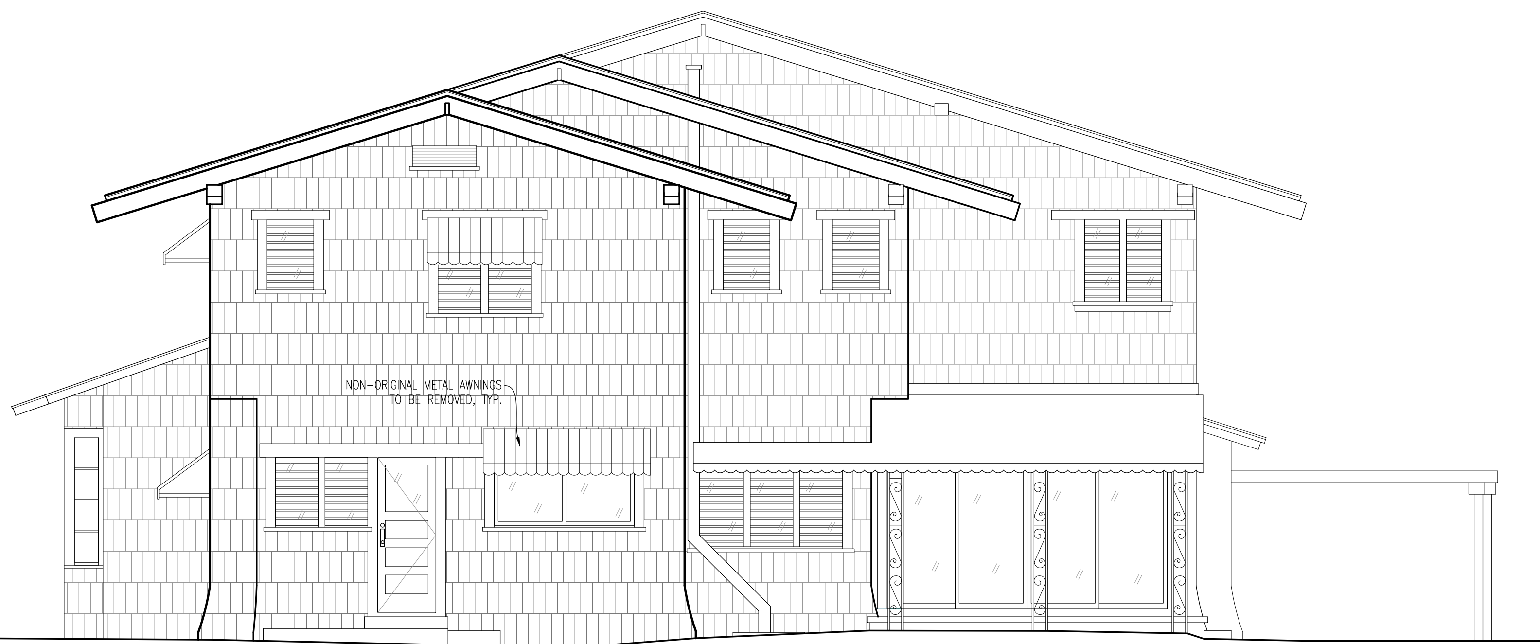
3 EXISTING SOUTH ELEVATION A-5 1/4" = 1'-0"
