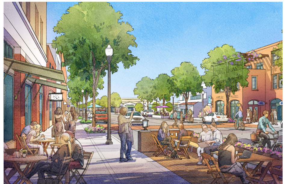
To augment pedestrian activity and social interaction along Mission Street, and to provide more sidewalk space, the plan proposes a series of parklets that occupy the space of one parallel parking stall, and are designed as intimate places for outdoor seating and dining.
