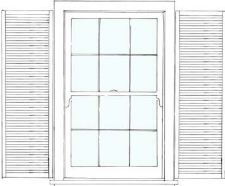
Window shutters may be found on Monterey Revival style residences. They are not appropriate on other Mediterranean and Indigenous Revival style residences.
