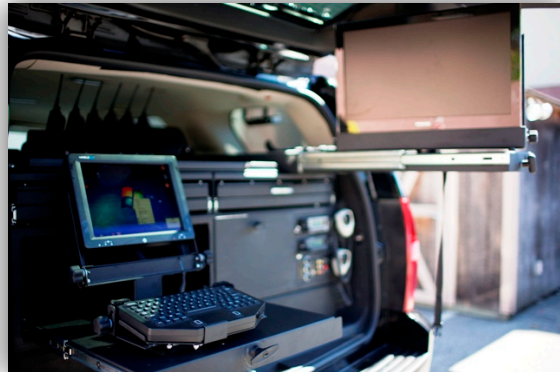
The Watch Commander's vehicle (Chevy Tahoe) is specially equipped to assist patrol officers in the field. The vehicle has spare radios, batteries, computer and a video down link system. The video down link works with air support, which enables patrol officers to get an aerial view of the scene.
