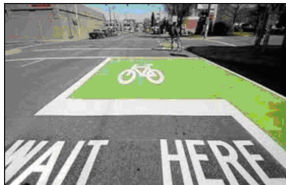
Figure 8.18 Bicycle Box Example (Portland)
